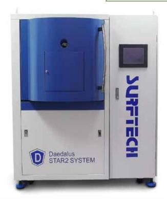
The SurfTech PVD (Physical Vapor Disposition) coating machine significantly increases tool life span by applying a 0.0001" layer of hardened coating to the tool's surface.
